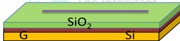
Figure 3: Single GaN-ZnO nanowire aligned between source and drain Ti/Au electrodes on SiO 2 /Si substrate.
